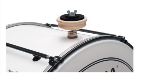
All cymbal holders feature a special interior insulator that avoids direct contact from cymbal to fixing screw – eliminating bothersome noise and vibration. The cymbal is fixed by a self-locking wing nut which will hold tight even when the cymbal is only loosely attached.
